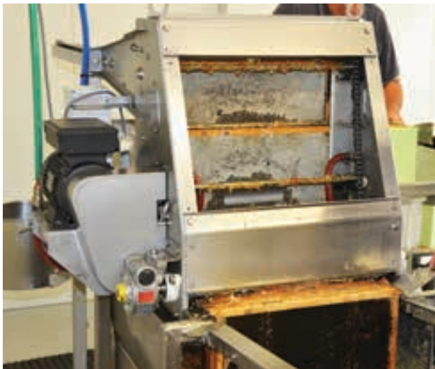
An uncapping machine. On the bottom right hand side of the photo an operator (not in view) uses a paint scraper to remove burr comb from the top bars of the uncapped frames and combs. The uncapped combs appear on the rack at the bottom of the photo.
