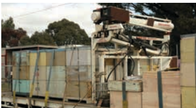
Split boom loader. Note the careful use of tie down straps and ropes to secure the load.
