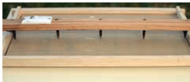
Electric embedder in use. Place all five studs of the embedder on the wire and carefully apply gentle pressure. Too much force may cause each heated wire to cut through the sheet of foundation.
