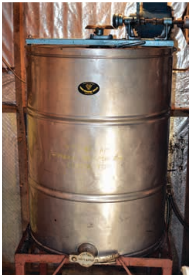
A 4-frame, stainless steel, electric driven extractor on stand.
