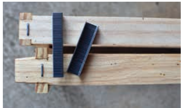
Staples are an alternative to nails.
