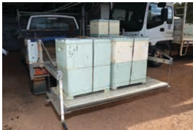
This manually operated tailgate lifting device easily lifts these hives.
