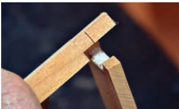
Glue all frame joints before nailing.
