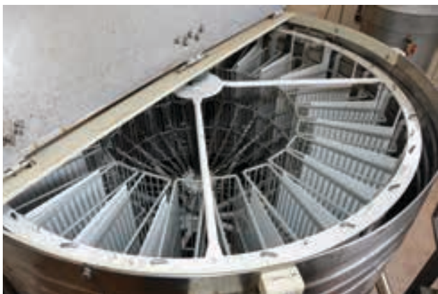
A 24-frame semi-radial stainless steel extractor.
