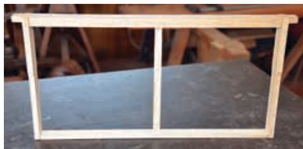
A well-fitted centre post glued between the top and bottom bars will give the frame added strength.
