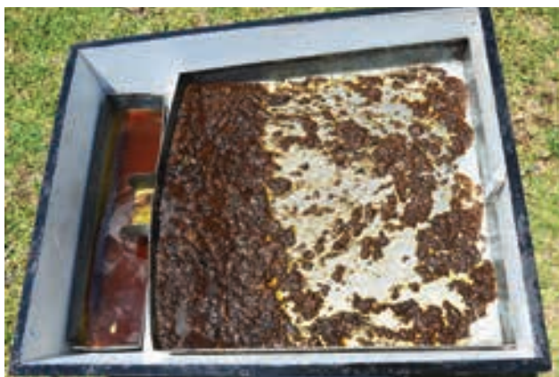
A solar wax melter in operation. The molten wax flows into the metal mould on the left. (The glass lid has been temporarily removed for this photo).
