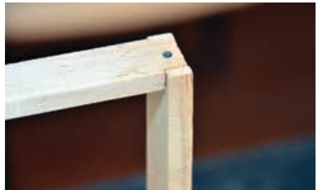
Nail the bottom bar first using one nail.
