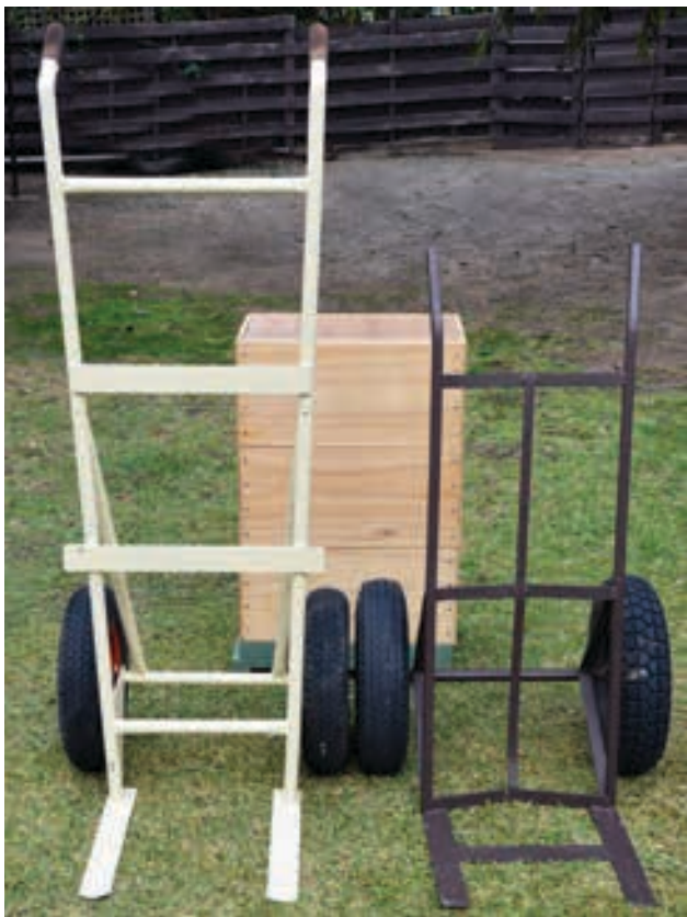
Hand trolleys suitable for moving hives. Note the large diameter wheels.
